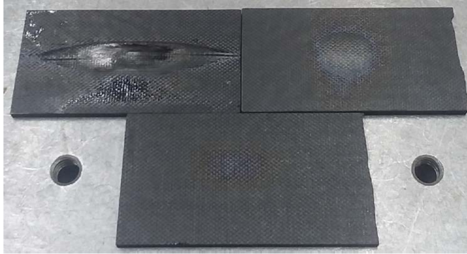
Figure 28. Top Left, sample 1.1 with fibers along the long axis of the beam. Top right, sample 1.3 with fibers orthogonal to the long axis of the beam. Bottom, sample 1.5 with fibers 45 ° to the long axis of the beam.
