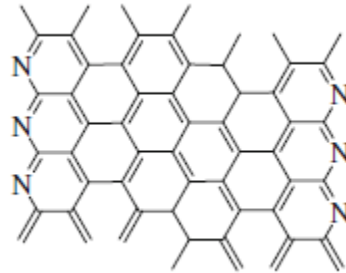
Figure 6. Resulting graphitic structure after carbonization and graphitization [22].
